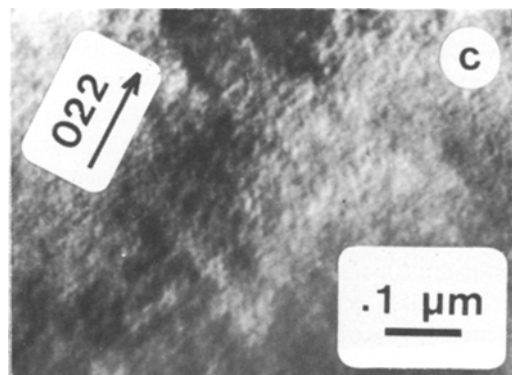
Figure 10 Tetragonally distorted structure obtained after 3 months' ageing at room temperature; (a) SADP, [100] zone axis, (b) enlargement of the (002) reflection, (c) BF image ( g = (022) , zone axis near [110] ), shows contrast striations parallel to \{110\} traces.
